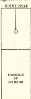
A simple homemade retinoscope, made by scratching a small hole in the silver back of a small mirror, to be used for self-testing in conjunction with another larger mirror.
