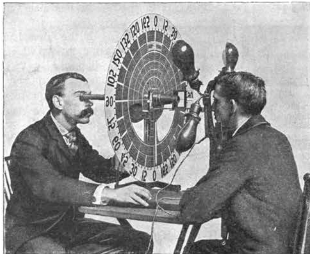
The Javal-Schiötz Ophthalmometer
